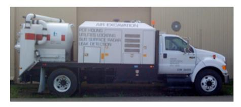
Potholing and Keyholing is more specifically known as SUE (subsurface utility engineering). It is the only way to know exactly where buried utilities are. Hawaii Geophysical Services is the only utility locating company in Hawaii to utilize this technology. We use a vac truck that employs air to excavate. Using air means there is no waste. The excavated earth can be placed right back into the hole. Hawaii Geophysical Services utilizes keyhole technology to pothole.
